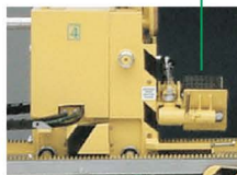
Main carriage with bundle locking system
